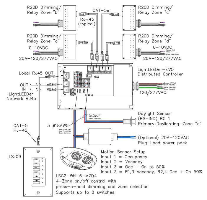
LightLEEDer EVO 4—Zone panel with 4—remotly mounted R20D relays Daylight sensor with independent zone settings, Motion sensor inputs for up to 4 independent zones or local hardwire switch. Optional plug—load relay. Local LightSync output for Multi—Zone Dimmer station (MZD) with raise/lower press—n—hold dimming, supports from 1 to 8 LightSync input devices.
