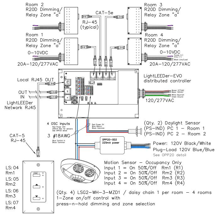
LightLEEDer EVO 4—Zone panel with 4—remotly mounted R20D relays Daylight Sensor w/ Independent zone settings, Motion sensor inputs for up to 4 independent zones or local hardwire switch. Optional Plug—load relay. Local LightSync output for Multi—Zone Dimmer station (MZD) with raise/lower press—n—hold dimming, supports from 1 to 8 LightSync input devices. Optional PC3—D3 & PC4—D4 as remote mount LS—PSC—IN (LS:08, 09)
