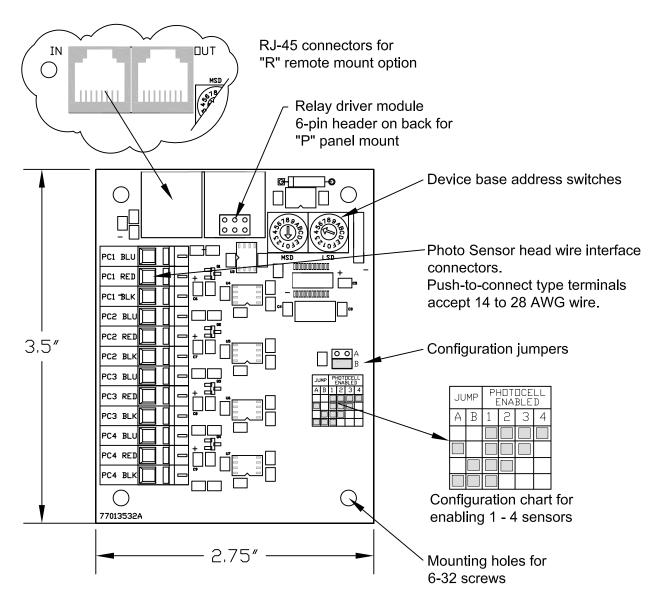
The LightSync Photo Sensor 4 module can be configured for 1 to 4 independent LightSync photo sensor devices. Place the configuration jumpers on A and B for the desired count.
