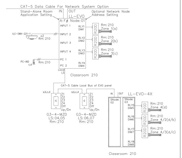
OPERATION: Switch ON/OFF On Level set for 50% dimming Motion sensor set for Vacancy Photocell limits max level in daylight zones
