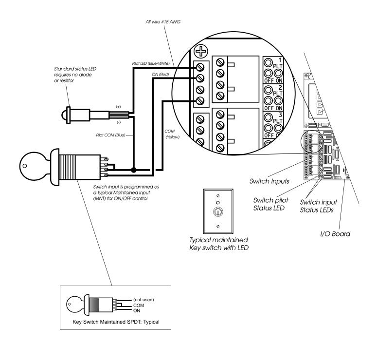
Typical Maintained Key Switch 2-Wire Wiring
